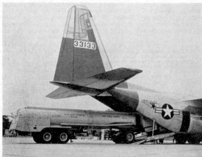
The Hercules can carry a U.S.A.F. type F-6 5,000-gall. fuel tanker and tractor in its 66 ft. long cargo compartment.
