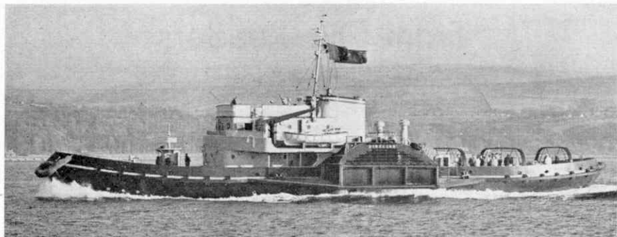
The "Director," the first of seven new Admiralty diesel-electric paddle tugs to go into service. Photograph by courtesy of Yarrow and Company Limited, Scotstoun.
