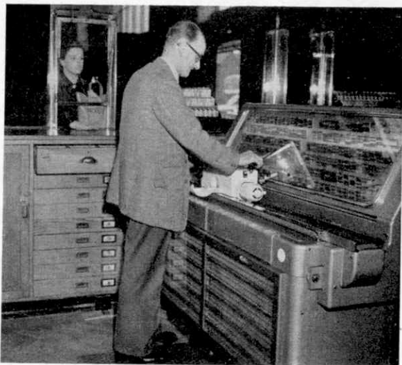
Issuing a ticket from one of the three recently installed machines at Doncaster. Each machine can print up to 1,260 different tickets, and it also adds up the receipts. B.R. (Eastern Region) photograph.
