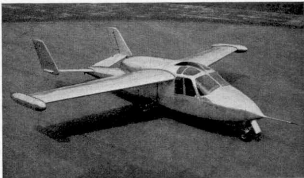
The Miles M.100 Mk.1 Student, which made its first flight on 14th May last. The wing span of this turbojet aircraft is only 29 ft. 2 in.
