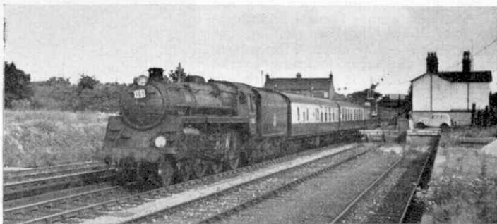
B.R. Standard 4-6-0 No. 73085 with an up Ramsgate train passing Sole Street station, near the summit of the incline of the same name. This route is referred to in the special article on pages 427-9. Photograph by S. Creer.
