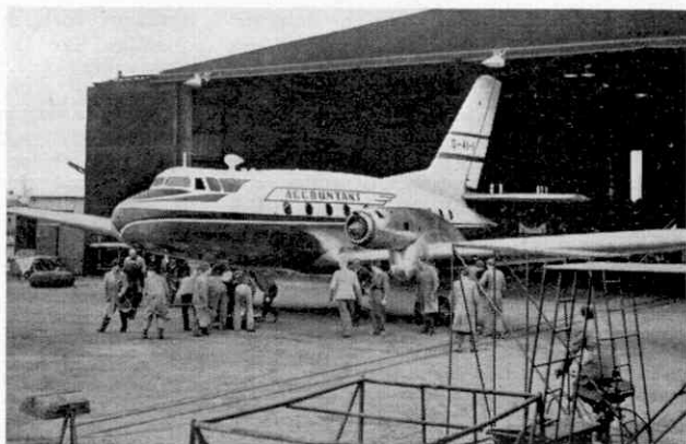
The prototype of Aviation Traders' Accountant transport being wheeled from the hangar. It will be noticed that at this stage the propellers had not been fitted.
