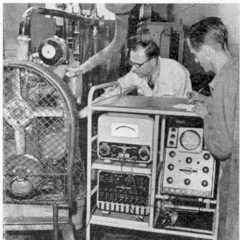
A test in progress with an engine running at full load. The curve on the screen on the left of the instrumental equipment tells the research engineers how parts in the engine are behaving.
