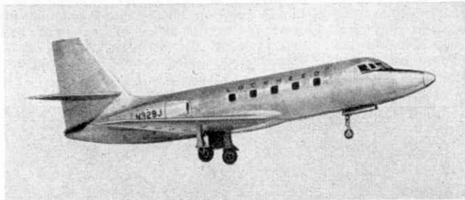
The Lockheed JetStar prototype in the air. The two turbojets are mounted in pods on the side of the rear fuselage.
