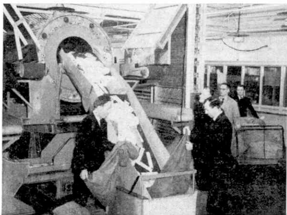
The loading end of a machine that automatically separates thin letters from newspapers, packets and bulky letters, and is described on page 158.
