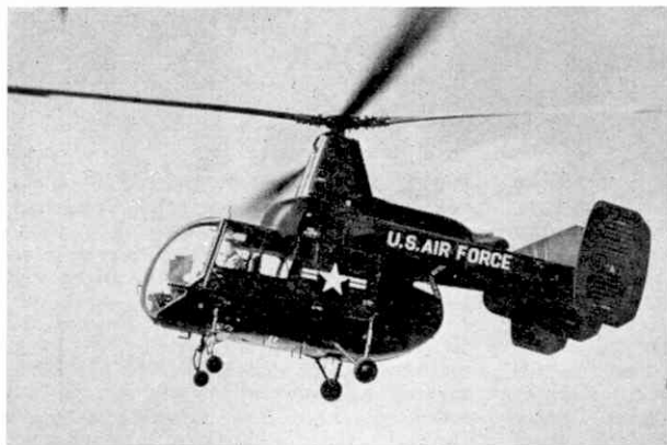
The Kaman H-43B, one of two versions of a crash-rescue helicopter ordered in quantity by the U.S. Air Force. This version is turbine-powered. Illustration by courtesy of Kaman Aircraft Corporation, U.S.A.
