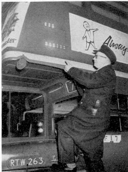
A driver points to the reflector on the side of his bus that will tell the control centre where it is when in service. Photograph by courtesy of London Transport.
