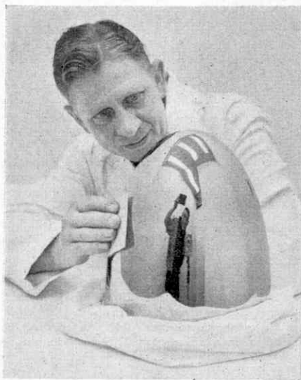
A blunt nose cone for use at speeds up to 10 times that of sound in the rarified upper atmosphere. Lockheed photograph.
