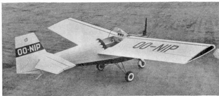
This Belgian ultra-light, single-seater aircraft is the Tippy Nipper, produced by Avions Fairey, of Gosselies.
