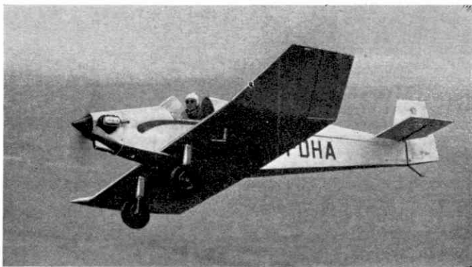
A successful ultra-light aeroplane introduced in the late 1940's is the French single-seater Jodel Bébé, which can be built up from a kit of parts.
