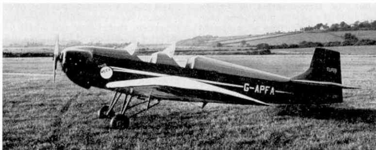
Perhaps the most popular of the "build-it-yourself" aeroplane designs sponsored by the Popular Flying Association is that of the single-seater Druine Turbulent. A two-seater version, called the Druine Turbi, is shown in this illustration.
