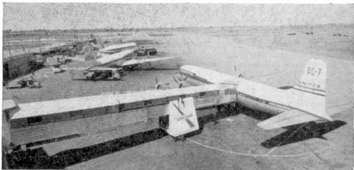
Positioned between aircraft and terminal building, United Air Lines' enclosed "Aero-Gangplank" provides a weather-shielded walkway for deplaning or boarding passengers at O'Hare Airport, Chicago.
