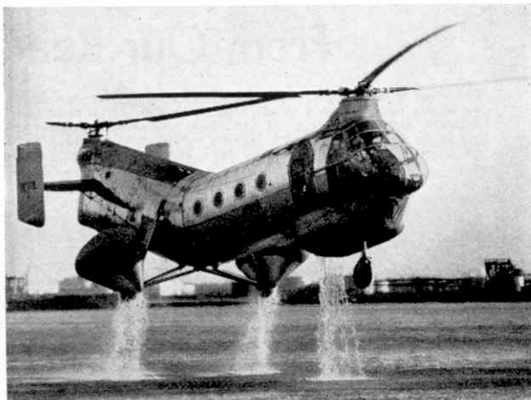
Vertol 44 tandem-rotor helicopter taking off from a river. The water is pouring out of the little cages that protect and shape the aft floats and from the fairing around which the forward float fits.
