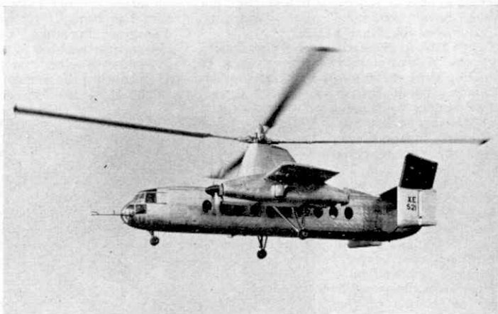
This view gives a good idea of the great sweep of the Fairey Rotodyne's powerful 90 ft. diam. four-bladed rotor.
