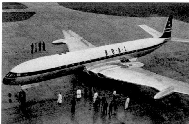
G-APDA, the first of 19 de Havilland Comet 4's for British Overseas Airways Corporation. It is half as large again and twice as powerful as the earlier Comet.
