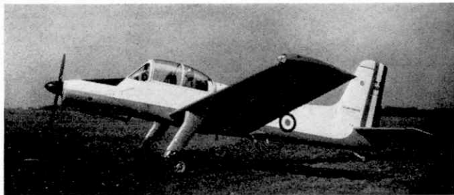
The new Morane-Saulnier M.S.1500 Epervier, a two-seat general-purpose observation and ground-attack aircraft. It has a fixed undercarriage.
