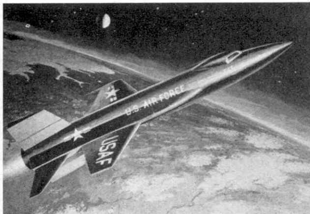
An artist's impression of the North American X-15 research aircraft described on this page. It is designed to fly at speeds of 3,500 to 4,500 miles per hour and at heights up to 100 miles.
