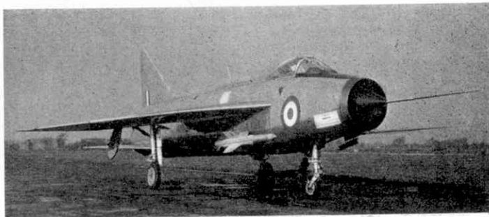
English Electric P.1B interceptor armed with two de Havilland Firebreak air-to-air missiles, one on each side of the fuselage.
