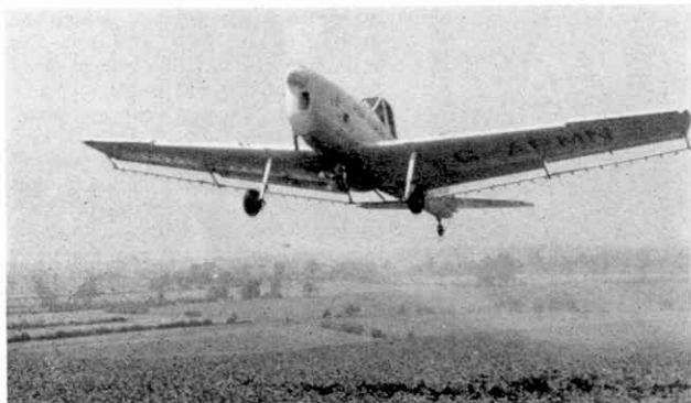
The agricultural version of the Chipmunk Mk. 23 aircraft can be used for either crop-spraying or dusting.
