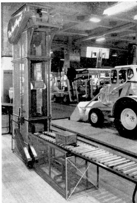
Fig. 1. The VertiVeyor shown set up for display purposes. The illustration shows the feed-in conveyor in the foreground. One load is being elevated on the swing tray, another is in position ready to be picked up while a third is being held back by the interrupter mechanism.
