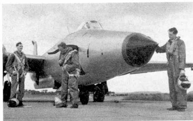
This Canberra aircraft was modified to provide a test bed for Airpass, enabling flight trials to be continued in conditions as near as possible to those in the P.1B.
