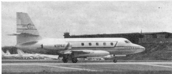
Lockheed JetStar transport, with two 300 gall. external fuel tanks fitted to the wing, increasing its range from 1,730 to 2,280 miles.
