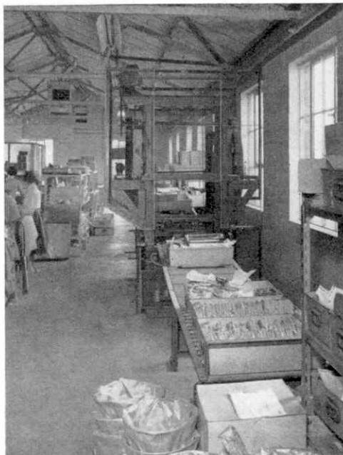
The VertiVeyor in action in a Factory, showing the "feed out" section of the installation in the foreground. Photograph by courtesy of Messrs. J. Collis & Sons Ltd., London.
