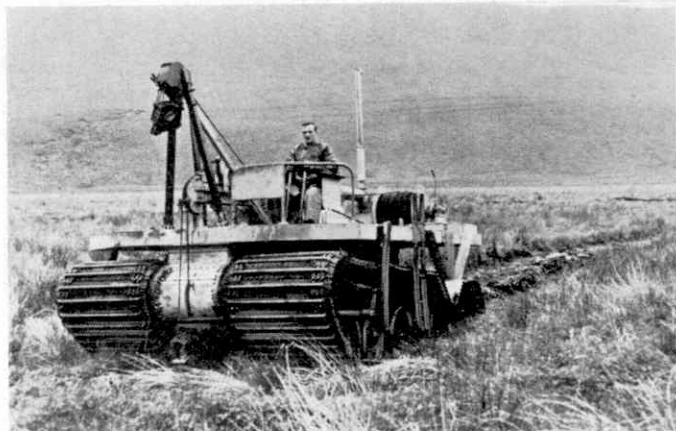
The Water Buffalo, a giant 20-ton tractor designed to travel over treacherous swamps. Shell photograph.
