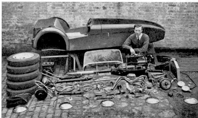
Kit of parts laid out, prior to assembly of a Lotus Seven in Basic trim. Assembly takes less than twelve hours.
