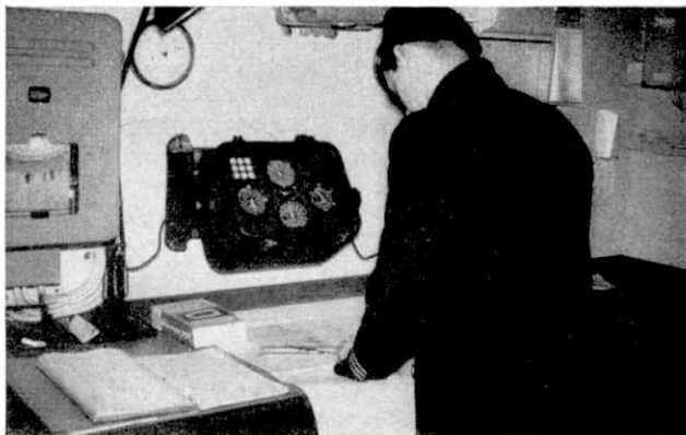
In the Chart Room of the tanker. On the left is the echo sounder and in the centre the Decca Navigator.
