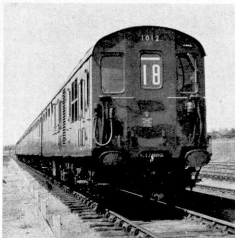
A head-on view showing the driving end of a motor coach on one of the 6-car diesel units used on the Hastings route. B.R. (Southern Region) Official photograph.
