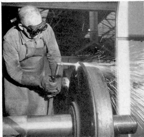
An oxy-acetylene burner cutting through the tyre of a wheel returned to the Acton depot of London Transport for servicing. Great care has to be taken that the wheel centres are not damaged by heat.
