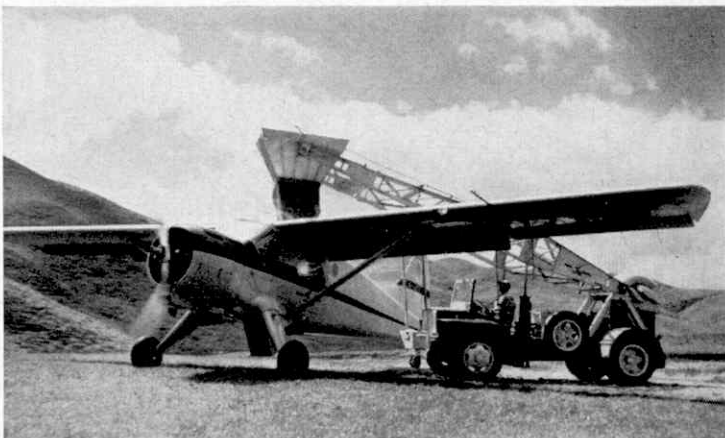
New Zealand leads the world in aerial farming. This picture shows a de Havilland (Canada) Beaver of Rural Aviation Ltd., New Zealand, being loaded with fertiliser, for spreading over barren hill country near Wellington. The fertiliser will be discharged from a hopper inside the cabin and will help to make the land suitable as pasture for sheep and cattle. Illustration by courtesy of the High Commissioner for New Zealand.
