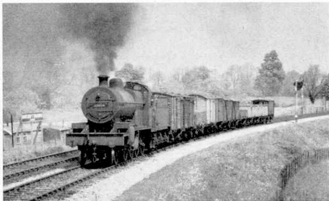
Ascending an incline of 1 in 60 between Chilcompton and Binegar, 2-8-0 No. 53804 passes Moorewood sidings with a light freight train.
