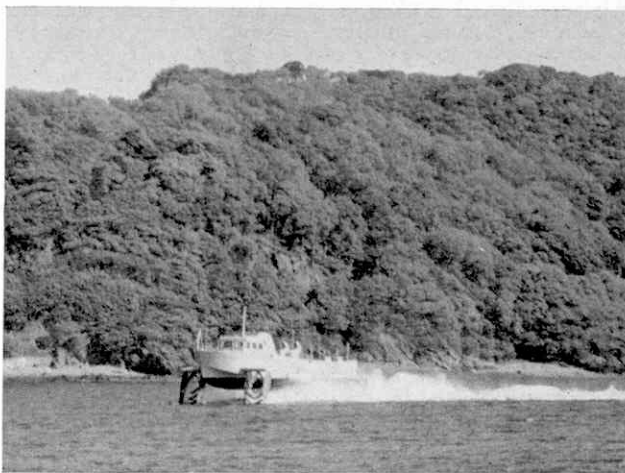
“Bras d’Or”, the Saunders-Roe hydrofoil craft at speed during trials. Note how the hull of the boat is lifted out of the water. Photograph by courtesy of Saunders-Roe (Anglesey) Ltd.
