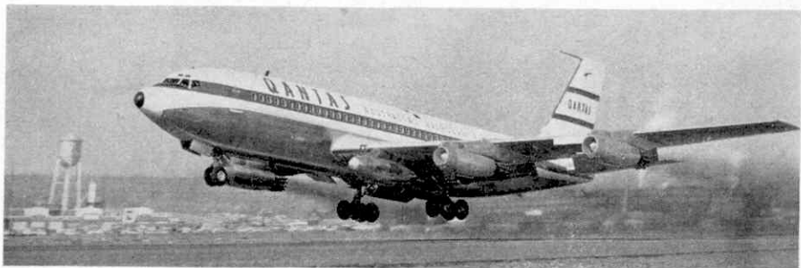
Boeing 707-138 jet-liner, with spare engine in a "Pod-Pak" under the port wing-root. This particular aircraft is in service with Qantas Empire Airways.
