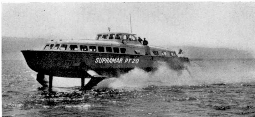
The Supramar hydrofoil vessel travelling the first with only its hydrofoils immersed in the water. Photograph Supramar A.G.
