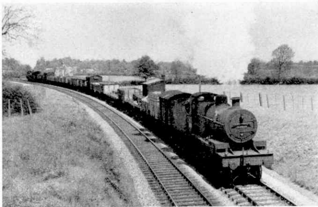
Ex-Somerset and Dorset 2-8-0 No. 53801 at Masbury summit, the highest point reached in the Mendips by the line, with a down freight banked by 0-6-0T No. 47557.
