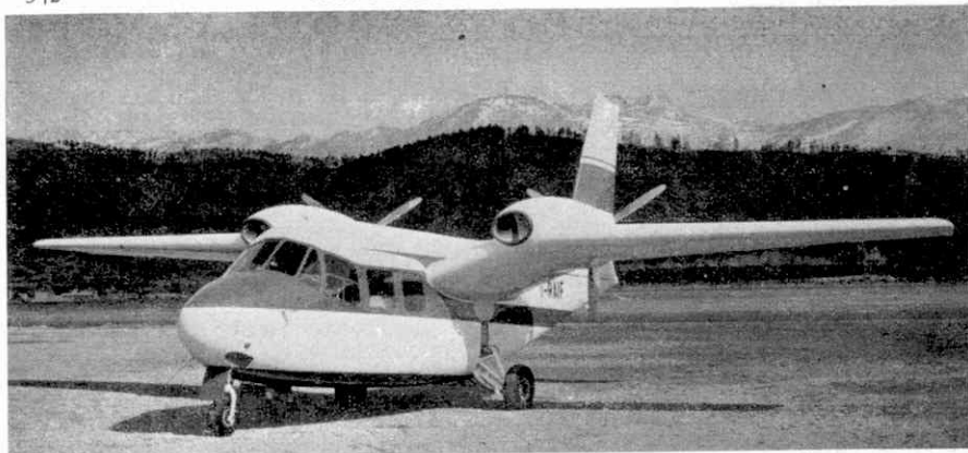
The Piaggio P.166, an interesting Italian pusher-type aircraft that can carry a pilot and seven passengers. Photograph by James H. Stevens.
