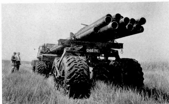
A Bedford 4 x 4 lorry and a Dyson Trailer loaded with oil pipes on Romney Marsh. Both lorry and trailer are fitted with low-pressure Terra-Tyres. Shell photograph.
