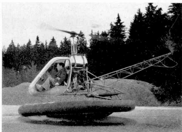
The German Bo 102 helicopter trainer is designed to "do everything but fly".
