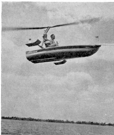
Aloft in a Bensen Gyro-boat, towed by a fast motor-boat.
