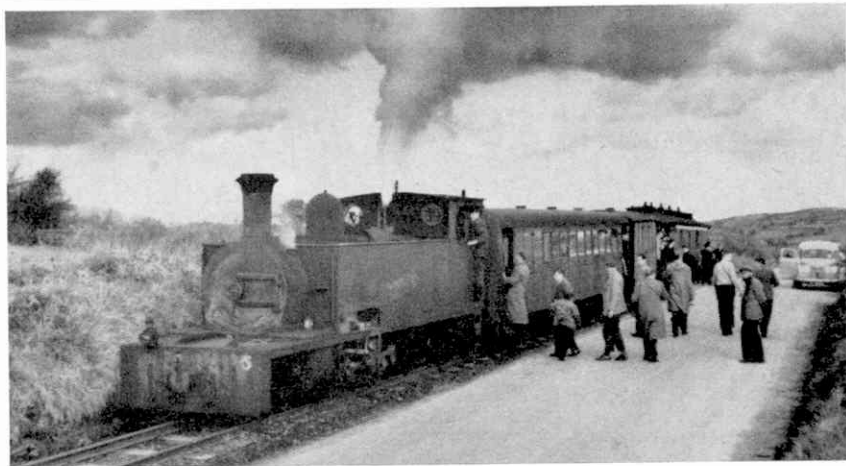
A roadside stopping place, with ex-Tralee and Dingle 2-6-2T No. 5T at the head of the train. The vehicle next to the engine was converted from two bus bodies.
