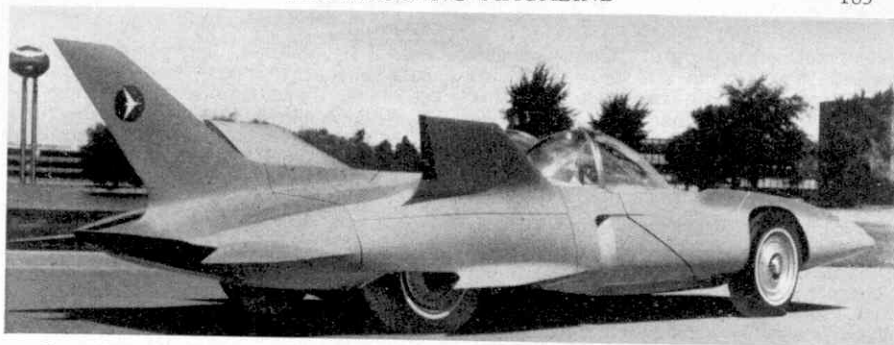
General Motors' newest experimental car, Firebird III. The main engine is behind the passenger compartment.
