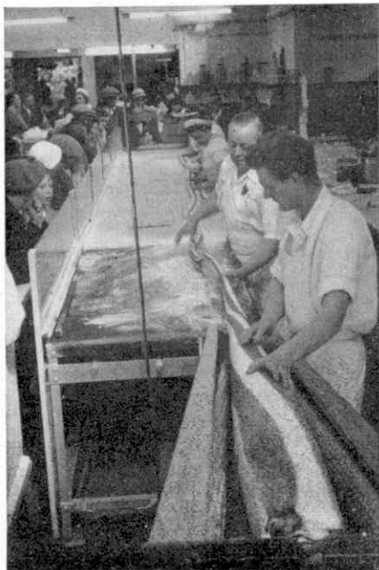
The cylinder is eventually spun out to the standard thickness required and cut into lengths.
