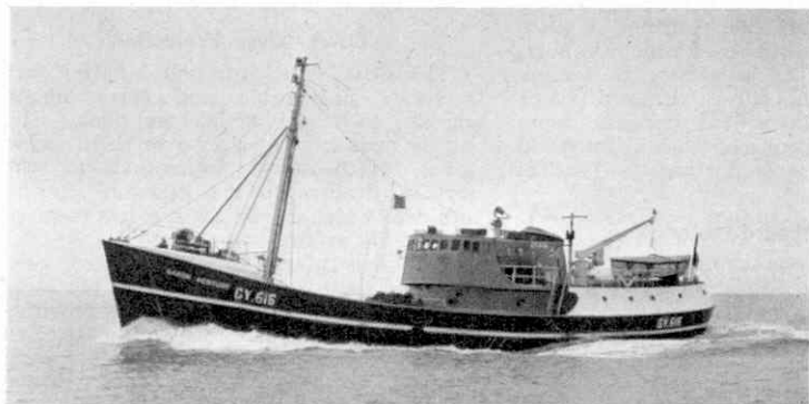
"Saxon Venture". A "Middle Water" trawler, 105 feet long and built by Richard Dunston Ltd. at Thorne, she fishes mostly in the North Sea.
