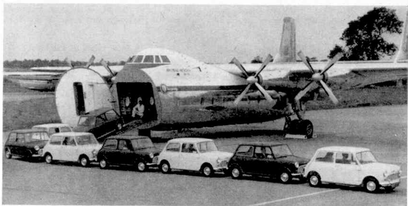
Morris Mini-Miror cars being unloaded from an Armstrong Whitworth Argosy transport aircraft.
