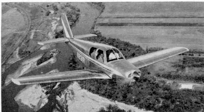
Beechcraft Debonair, an American four-seat lightplane with a cruising speed of 180 m.p.h. at 11,000 ft.
