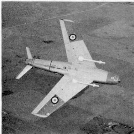
The first R.A.A.F. Sabre jet-fighter to be equipped with Sidewinder air-to-air guided missiles. They are clearly visible under the wings.
