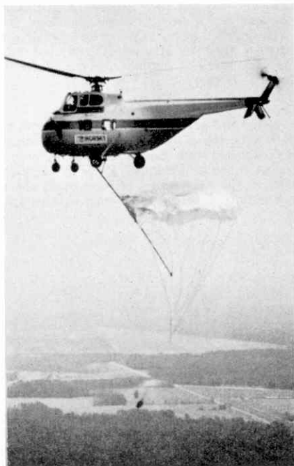
Picking up by helicopter a load suspended from a descending parachute. Here a Sikorsky S-55 snags the parachute shroud lines on a special hook at the end of a 20 ft. boom.
