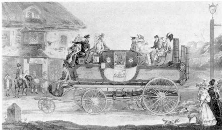
This print of Gurney's steam coach (1827) shows the engineer in front controlling the vehicle. The carriage was 15-20 feet in length and weighed about two tons. The rate of travel was intended to be from 8-10 miles an hour. Photo., Science Museum, London.
