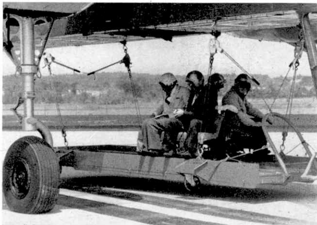
Sikorsky engineers buckle their seat belts as they prepare for an experimental flight on an open platform carried by the Sikorsky S-60 crane helicopter. Igor Sikorsky is on the right (facing camera).
