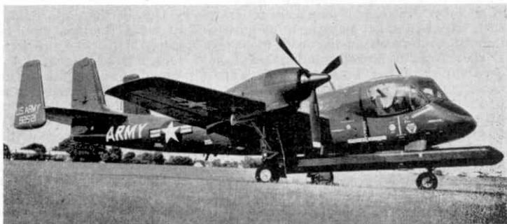
The Grumman Mohawk two-seater aircraft showing the SLAR equipment.
