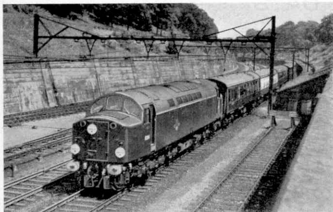
Type 4 diesel-electric locomotive No. D204 descending Brentwood bank with an up express from Norwich. Steam, diesel and electric trains traverse this stretch of main line, the overhead wire supporting structures being clearly shown. Photograph by S. Creer.
