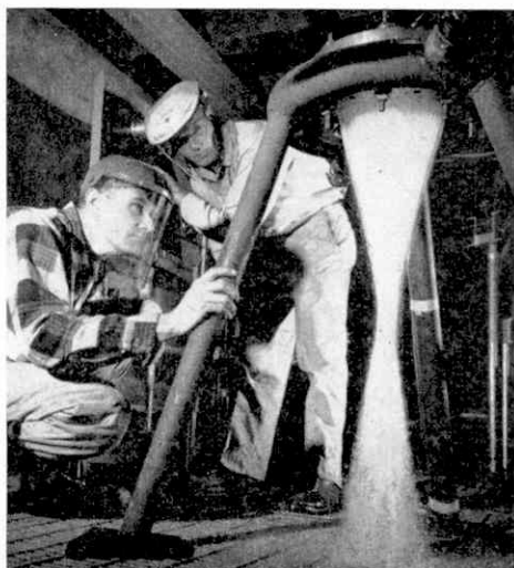
Fig. 2. Technicians inspecting the pattern formed by water flowing through the multi-hole injector of a 20,000 lb. thrust rocket engine. (Picture: National Aeronautic and Space Administration.)
