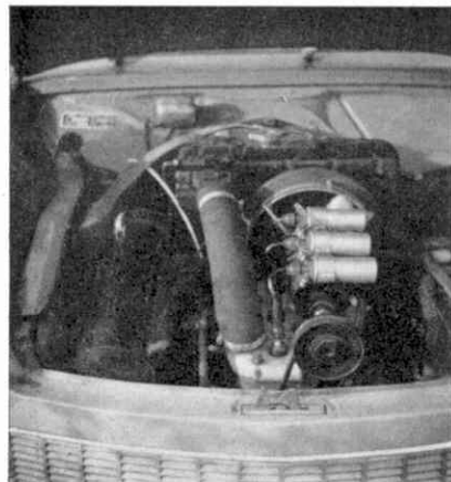
The engine of the D.K.W. Junior, with a separate ignition coil for each of the three cylinders.
