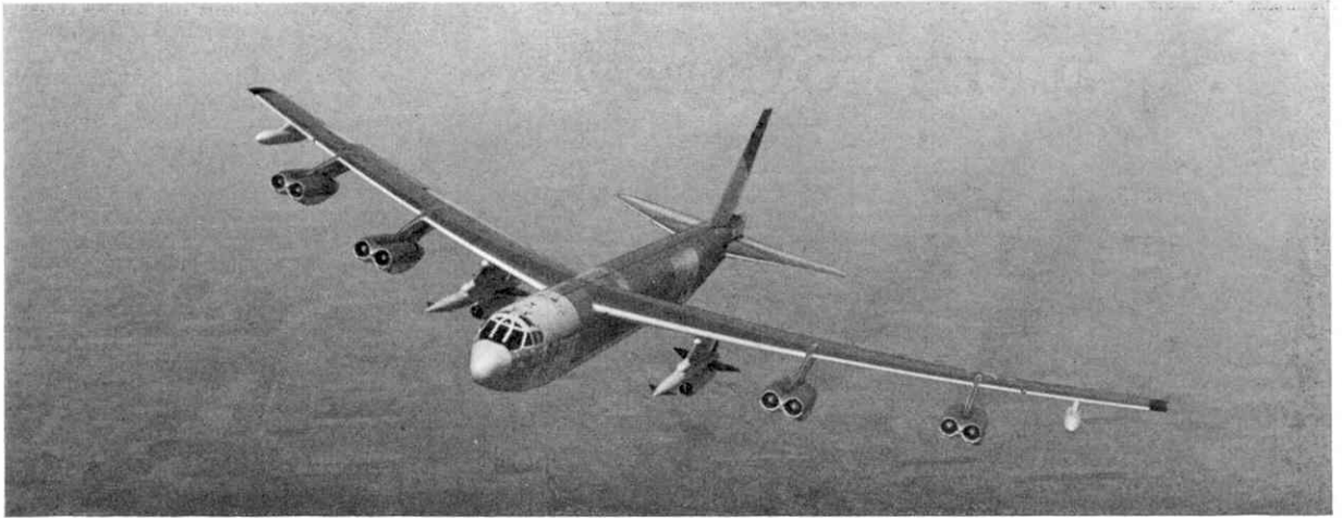
Carrying a Hound Dog under each wing the B-52G can release its weapons hundreds of miles from the target.
