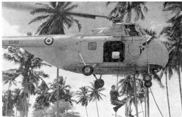
A Whirlwind helicopter from No. 110 R.A.F. Squadron picks up a soldier, clad in jungle green, in the Malayan jungle by means of a thick rope. This rescue method is used when a helicopter cannot use a landing zone.
