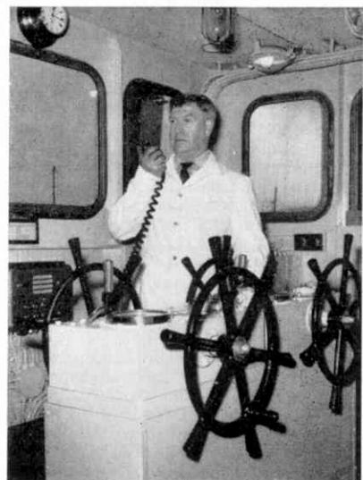
In the central wheelhouse the steersman is shown operating the Marconi talk-back system.
