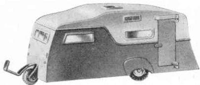
This view of the four-berth Caravan clearly shows the jockey wheel and towing bar.
