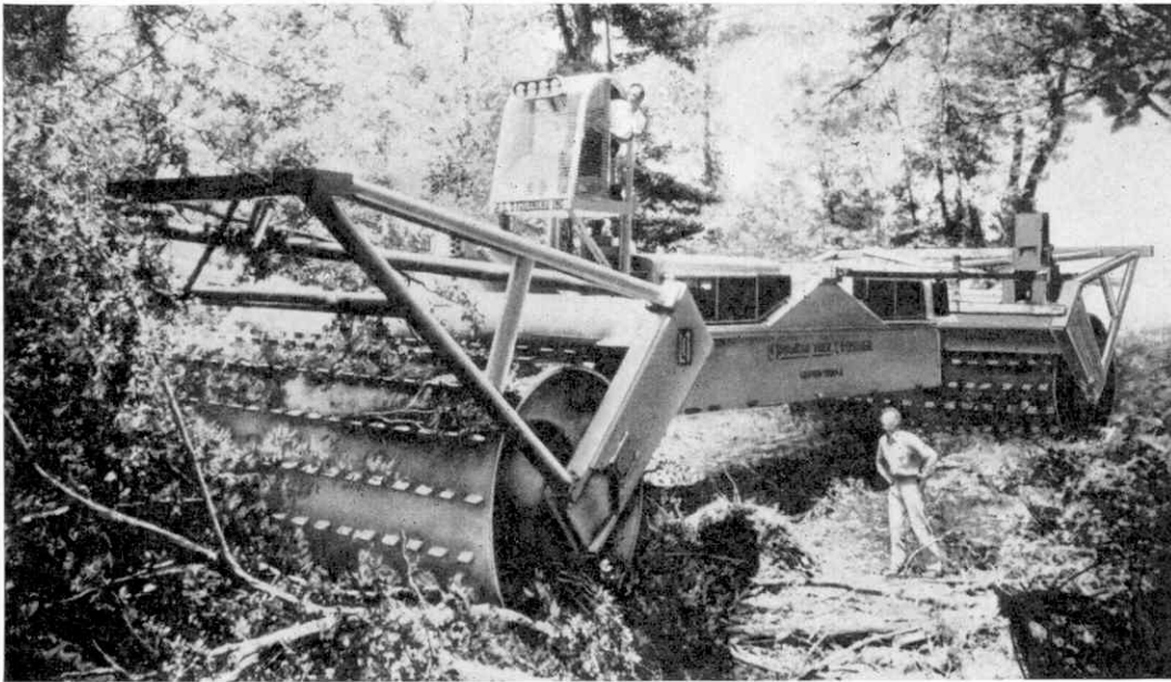
A tree-crusher is seen here tackling an area of unproductive forest land. The machine's operator is in the cabin on top, and in the right foreground is the job foreman.
