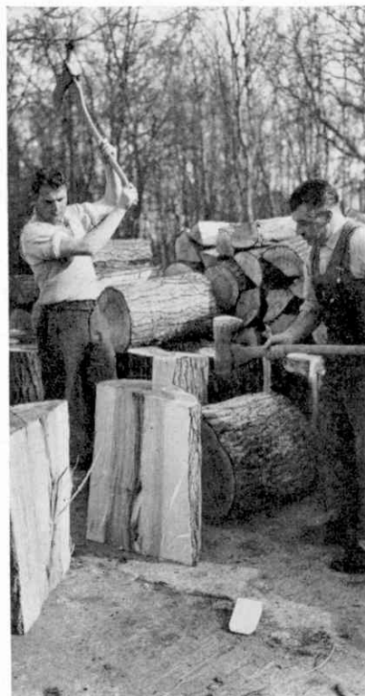
After being sawn into 28-inch lengths, the timber for cricket bats is split into “clefts”, each piece providing material for one bat blade. Splitting is done with an axe and calls for great skill.
