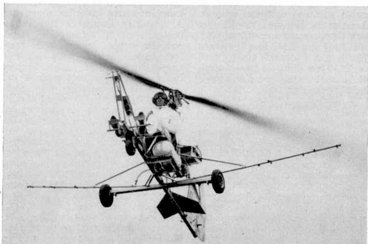
The Napier Agri-Copter agricultural gyroplane in the air. The spray-chemical tank is mounted behind the pilot's seat and feeds, by flexible polythene pipes, the spray booms extending on either side of the aircraft.
