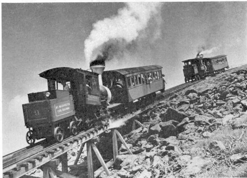
For more than 70 years these locomotives have been pushing coachloads of passengers to the top of Mount Washington. This illustration gives an idea of the gradients encountered on this fascinating railway line. Like the other photographs illustrating this article, it appears by courtesy of the New Hampshire State Planning and Development Commission.
