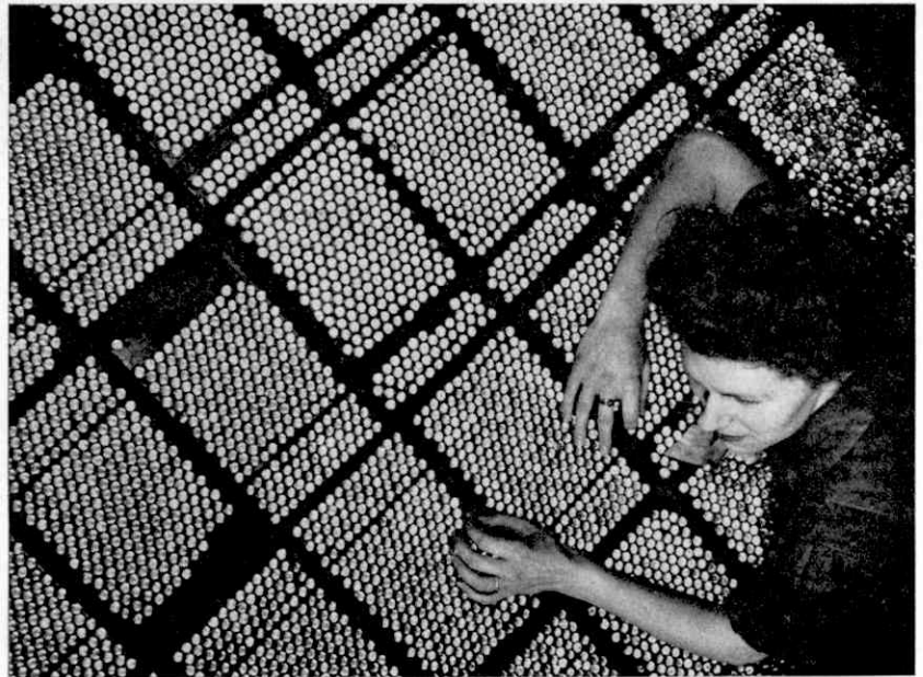
The brilliance of these reflecting lenses, which are being sorted before being installed in the rubber cups of the cat's eyes, makes this picture seem more appropriate to a jeweller's shop than a factory. Central Office of Information photograph: Crown Copyright reserved.
