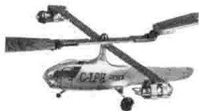
JET HELICOPTER Powered by two Jetex motors at rotor tips. Ascends 100 ft., descends by autorotation. Price complete 27/-.
