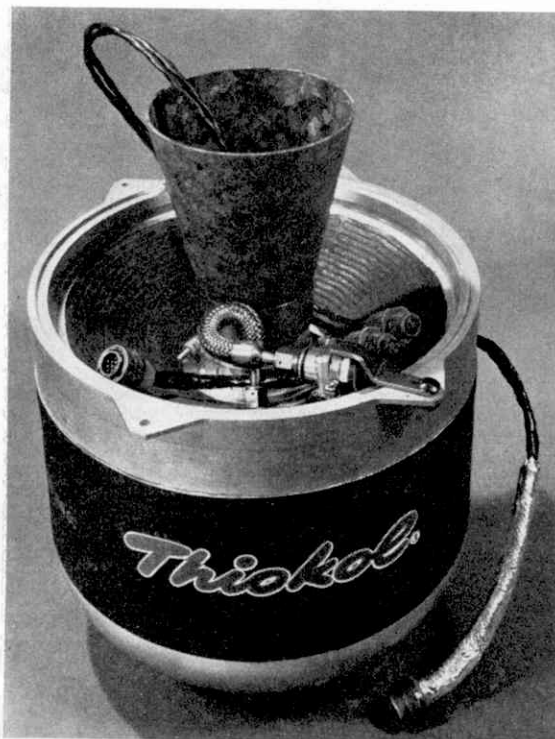
Above: Retrograde rocket engine for the Mercury manned capsule showing igniter leads and heater blanket. Three of these engines were used to brake "Friendship 7." Thiokol Chemical Corporation photograph. Right: Except for the balance wheel (marked with tiny holes) all parts of this space gyro are made of a virtually indestructible ceramic. Illustration by courtesy of Minneapolis-Honeywell Regulator Co.
