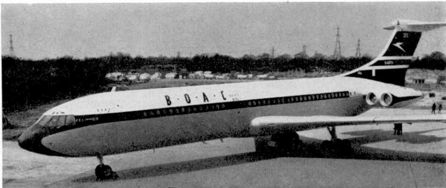
This photograph clearly shows one of the distinctive features of the VC10, the mounting of the 21,000 lb. Rolls-Royce Conway 42-1 turbojets in pairs on either side of the rear fuselage.
