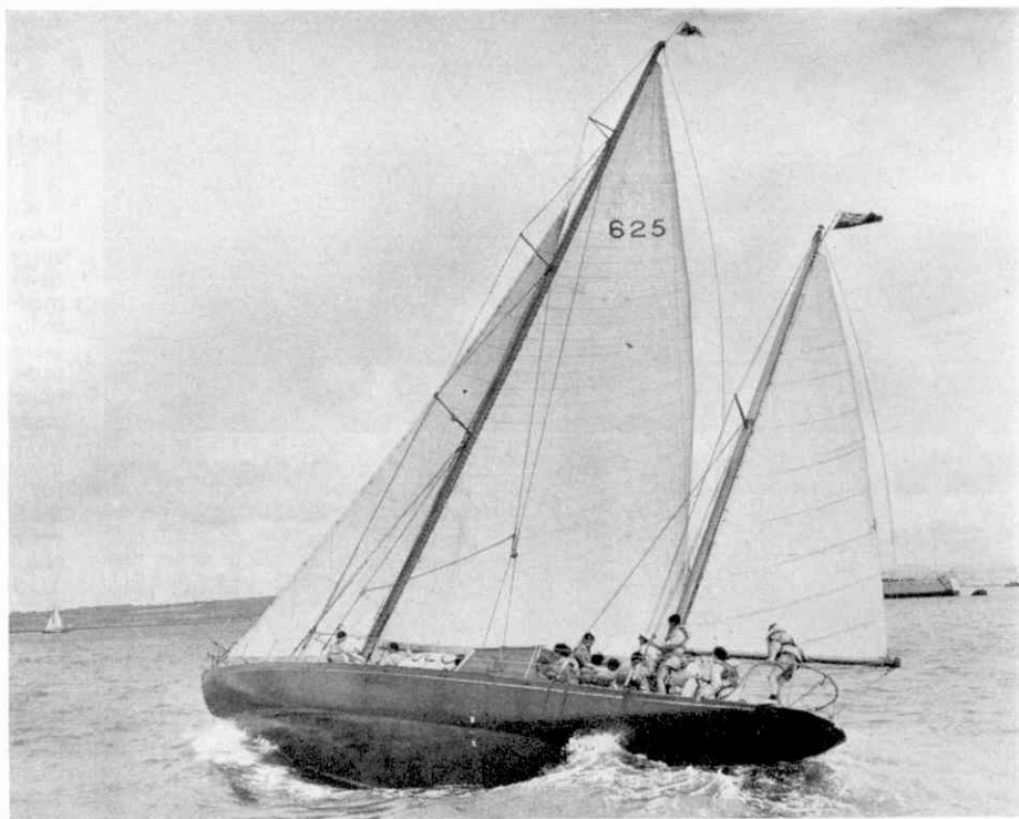
The ocean racing yawl "Marabu" (length overall 57.7 feet; load waterline 39 feet). Note the distance between the wave crests, which must be about 36 feet. This means she is travelling at a speed/length ratio of about 1.1, or about 7½ knots. She is, in fact, sailing on more than her load waterline.
