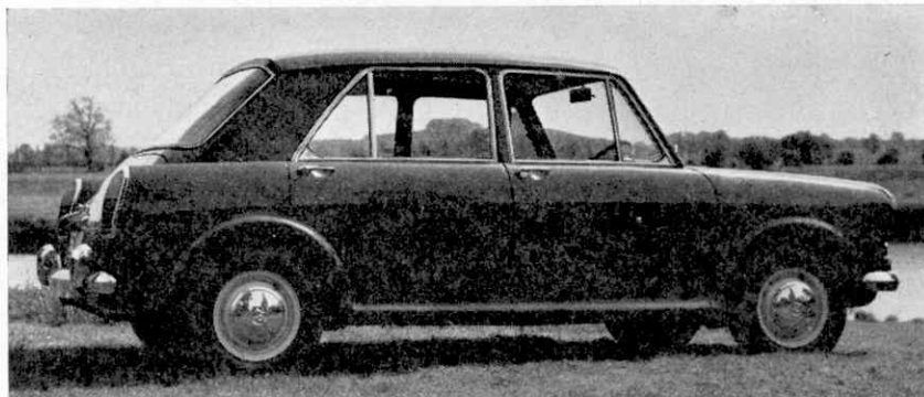
Transverse engine, front-wheel drive, independent hydroelastic suspension and disc brakes on the front are features of the new Morris 1100 pictured here.
