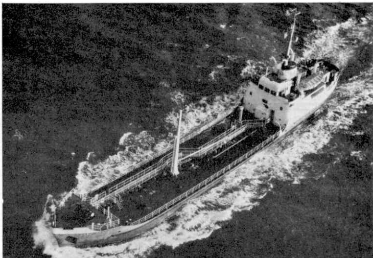
The catwalk and small hatches on the m.v. "Esso Ipswich" (1,103 tons) are clearly seen on this picture taken on the vessel's trials two years ago.
