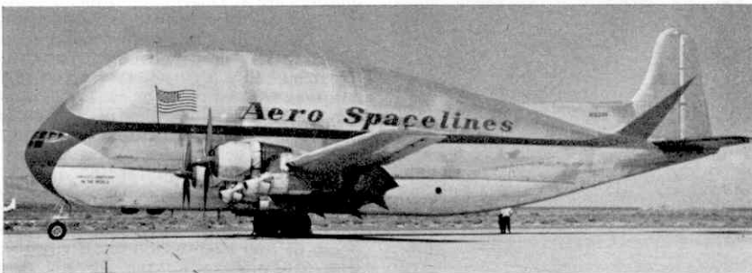
The Stratocruiser modified for Aero Spacelines Inc., U.S.A., by the On Mark Engineering Company to carry large booster rockets.
