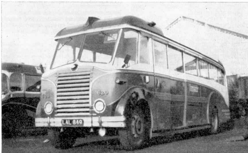
Barton's No. 620 (LAL 849) is certainly a rare bird, being a Leyland Comet CPO1 of 1949 vintage with a Beccols FC 34F body. Picture by N. J. Peel.
