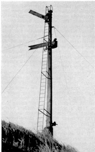
An L.N.W.R. signal post to which an upper quadrant semaphore has been fitted. Picture by W. S. Garth.
