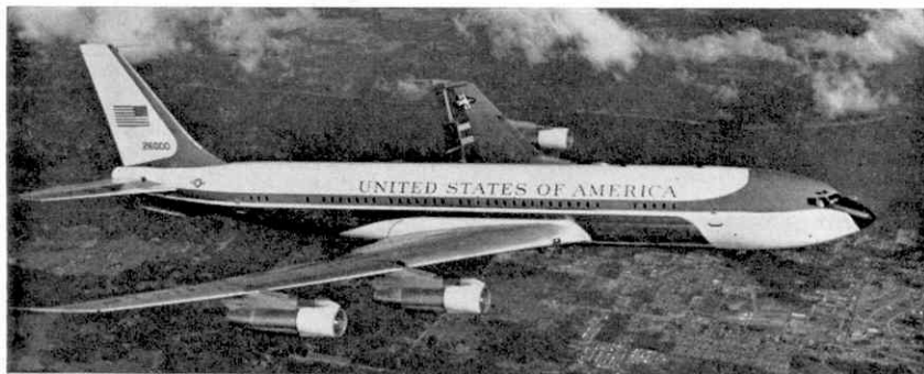
Intended to provide transport at over 550 m.p.h. for important members of the U.S. Government, including the President, is this specially-equipped Boeing VC-137C jet transport.
