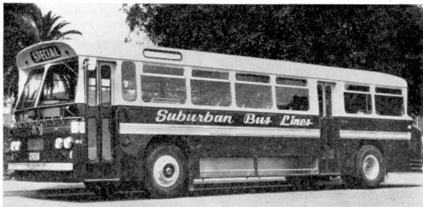
One of two 140 h.p. rear-engined Leyland Lions with 42-seater bodywork now being operated by Nelson Suburban Bus Co. Ltd., New Zealand. There is a baggage compartment on each side of the bus (one is clearly visible in the picture) and a rack at the front for carrying prams.
