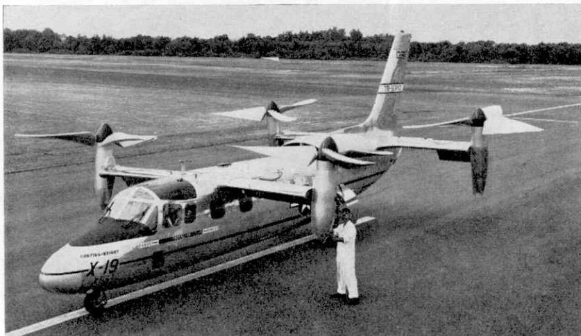
Top picture: The new English Electric Lightning F. Mk. 3 fighter with overwing fuel tanks for long-range ferry flights. Below: The Curtiss-Wright X-19A VTOL research aircraft, with "radial lift-force" propellers in take-off position.
