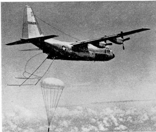
Left: A Lockheed JC-130B Hercules of the 6593rd Test Squadron, U.S.A.F. retrieving a Discoverer satellite in mid-air. The squadron is based at Hickam Air Force Base, Hawaii. Above: The prototype Dinfia Guarani II turboprop transport, built in the Argentine.
