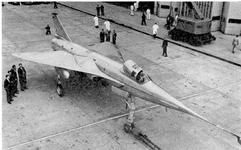
The BAC 221 single-seat research aircraft—first ever with wineglass-shape "ogee" wing.
