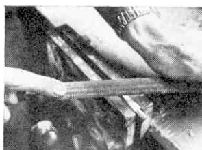
When all is screwed up hand tight and the locking ring has been positioned, the cranks can be refitted. New cotters are unlikely to fit straight away and must be filed until they fit properly.
