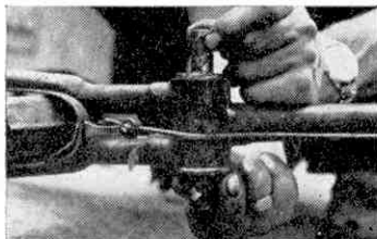
Fill the adjustable race with grease and lay it handy. Push the spindle into the bottom bracket from the top and holding it in place, turn the bike over. Now, as shown, the adjustable race can be screwed in from beneath.
