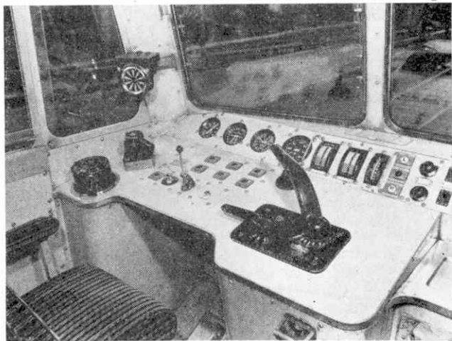
The cab of the 25 kV, 3,300 h.p. electric locomotive.
