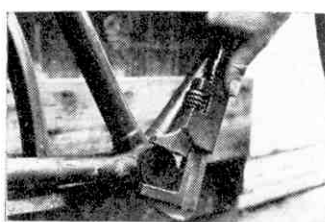
With this unscrewed, the bottom bracket spindle can be withdrawn and probably most of the ball bearings will fall out. The race on the other other side can be unscrewed using an adjustable spanner. The thread is left hand.
