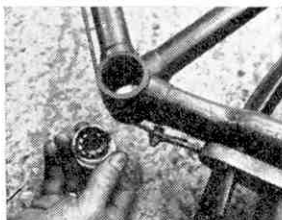
The new fixed race is wiped clean and filled with clean new grease. Eleven 1/2 in. ball bearings are carefully placed round the race. Lay the bike on the ground and screw the race in from underneath.
