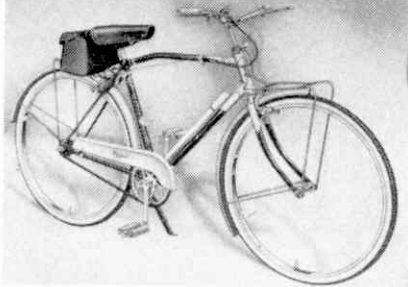
Another model in the Wearwell range is No. 59 Sports which has a 19½ inch frame and 26 by 1½ inch wheels. Costs £19 7s 6d.
