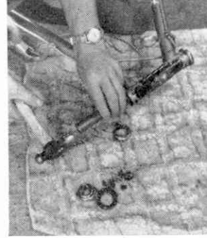
Clean up all the parts and inspect them for wear. If the lower races are worn, they must be renewed. Use a copper drift to tap them out.
