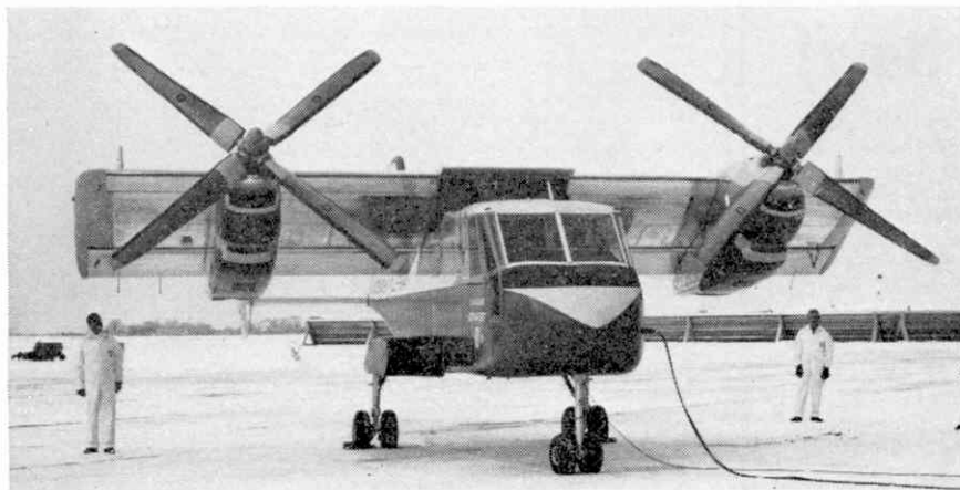
A tilting wing is the secret of the new Canadair V/STOL Dynavert
