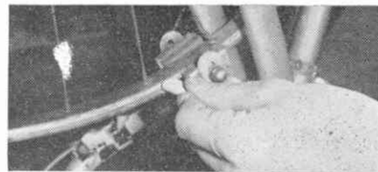
Fig. 2—Using a piece of chalk, steadied by the brake block to mark the buckled area on the rim. The chalk marks as the wheel spins. Tighten spokes opposite side of chalk marks and loosen on the same side as the mark.
