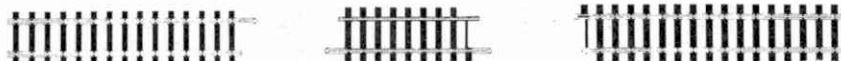
How a Converter Track connects Tri-ang Railways Super 4 with Hornby Dublo Track.
