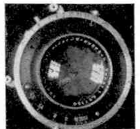
Cameras with between lens shutters have the shutter speeds marked around the outside, with a small pointer for setting the speed required. Note that with all shutters you must set directly on to the speed required. You cannot set between 1/50th and 1/100th and get a speed of 1/75th, you will only wreck the shutter. Top speed available on this type of shutter is normally 1/500th.
