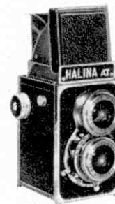
Cameras with between lens shutters have the shutter speeds marked around the outside, with a small pointer for setting the speed required. Note that with all shutters you must set directly on to the speed required. You cannot set between 1/50th and 1/100th and get a speed of 1/75th, you will only wreck the shutter. Top speed available on this type of shutter is normally 1/500th.
