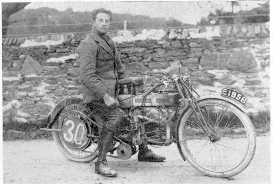
Believe it or not, but machines like this old twin-cylinder Douglas were actually raced in the T.T. This photograph dates back to 1913 and the rider was E. Elwell. Note the belt drive and stirrup-type front brake and large toolbox on the petrol tank to carry out running repairs
