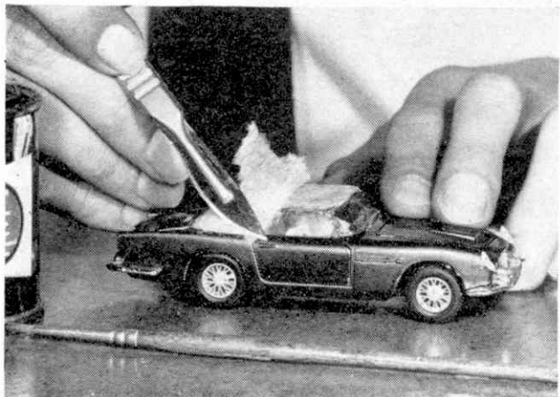
When the twelve layers of tissue and dope have dried hard, the moulding is peeled off the former, trimmed, and glued into position on the car with an impact adhesive. Any cracks remaining are then filled with tissue paper and dope, pressed into position by the modelling knife. When the final coating of dope has dried, the entire car can be painted, in this case with maroon, giving two or more coats until the original colour is completely obscured, and the new hardtop adequately coated
