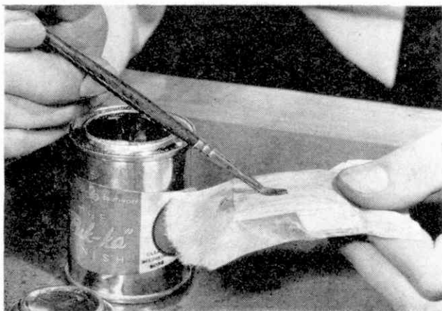
Once the surface of the balsa former is shaped, it is rubbed with wet soap and a piece of tissue paper is applied over. Small cuts are made in the tissue paper to allow it to conform to the curves on the former and it is given a coating of dope. The simulated folded hood behind the rear seats of the Dinky Toy model is then sawn off with a hacksaw and the upper edges of the sides and end of the seat are cut and filed until they are flush with the top of the side of the car
