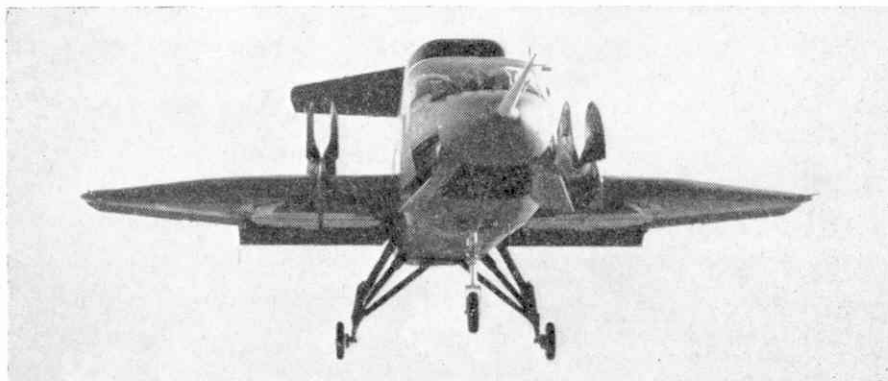
Three different views of the XV-5A. These show the louvres on the under-surface of the wing and the hinged doors on the upper-wing, the air deflectors on the nose, and a shot of the aircraft in flight
