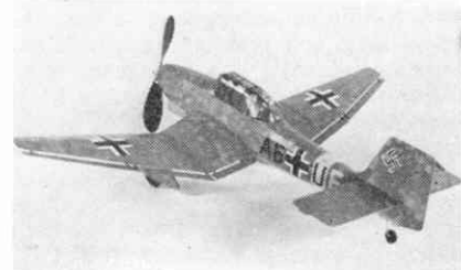
Junkers 87 by KeilKraft. The mottle finish was achieved with an aerosol using a cardboard "mask" as stencil
