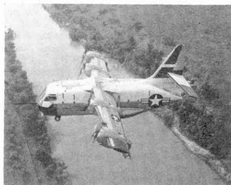
America's big 32-seat XC-142A military transport aircraft comes in to land, with its wings beginning to tilt upward for a vertical touchdown. The story of this 20-ton 'hummingbird' is told in a special article on pages 16 & 17
