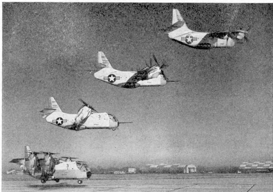
A composite photograph showing the wing movement necessary to achieve transition to forward flight
