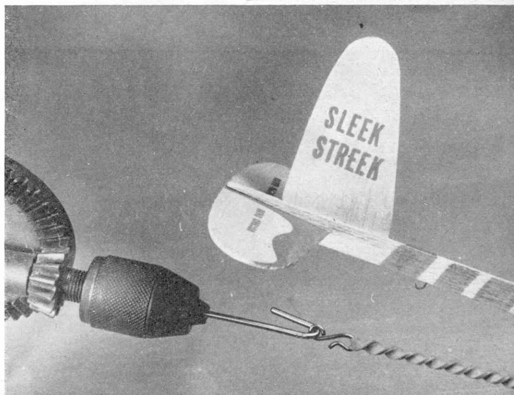
Photograph on the facing page shows Roger Davies with his Sleek Streek—just airborne and climbing fast! Above: four models that just clip together (the Astro-Gnat has no undercarriage). Right: marking the identification number on the rudder with a fibre tip pen. Below: an 'S' hook simplifies the re-attachment of a wound rubber motor
