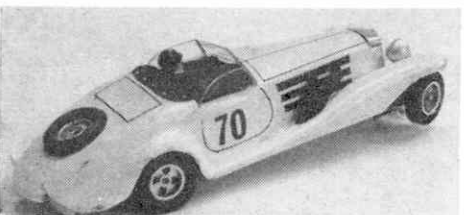
This Mercedes, belonging to a member of our slot racing club, has a hand-built wooden body and no chassis, the working parts being fitted directly onto the underside of the body.
