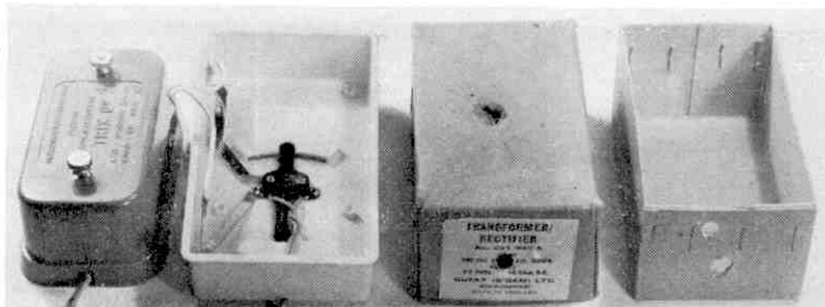
Above: The Beattie conversion of the Wrenn-Lima battery control box. This incorporates a Trix transformer and Wrenn switching system most effectively giving variable speed, forward and reverse controls for only 10s.
