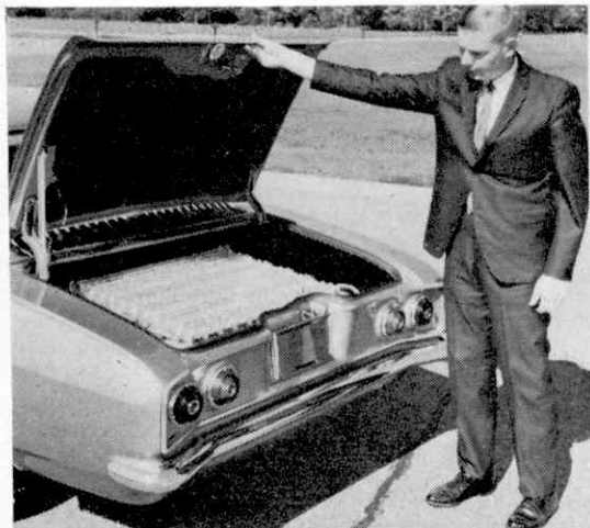
These front-and-rear views show the silver-zinc battery pack electric car built as a test bed for motor and control elements. Its performance is similar to a petrol powered Corvair, except for its 40-80 miles cruising range before recharge. A standard Chevrolet Corvair can travel 250-300 miles on a tank of petrol.
