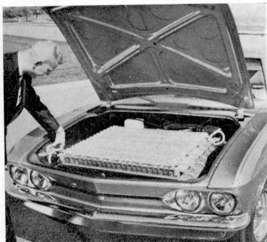
These front-and-rear views show the silver-zinc battery pack electric car built as a test bed for motor and control elements. Its performance is similar to a petrol powered Corvair, except for its 40-80 miles cruising range before recharge. A standard Chevrolet Corvair can travel 250-300 miles on a tank of petrol.
