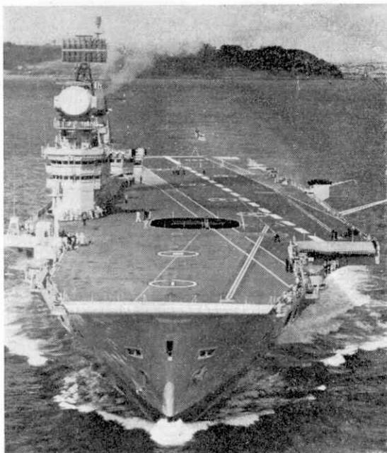
H.M.S. Eagle showing flight deck and hatch where the aircraft are brought up from the hangar. Ministry of Defence Crown Copyright photo.
