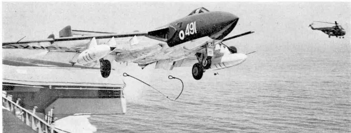
As this Sea Vixen Mk I takes off, the strop (by which it was connected to the steam catapult) falls away into the sea—this is not recovered. Note the 'plane guard helicopter hovering.
