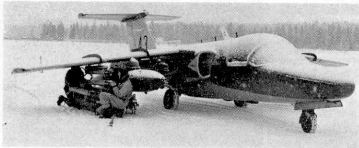
Ground crew members loading 13.5 cm. rockets under the wings of a SAAB 105XT which, in this arctic scenery at Vidsel, also carries two gun pods each housing one 30 mm. cannon.
