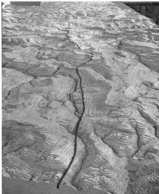
This model was used to assist in early location work. The proposed route of the new Motorway is shown running straight down the centre.
